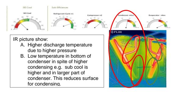
Figure 7, Air cooled chiller with too much refrigerant charge
