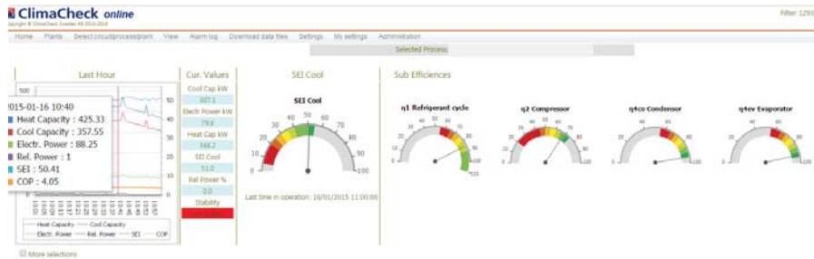
Figure 4.6 - SEI and Sub efficiencies can be visualised and impact of pumps and fans can also be expressed as efficiencies to benchmark performance on a component level and high light where measures are justified.
